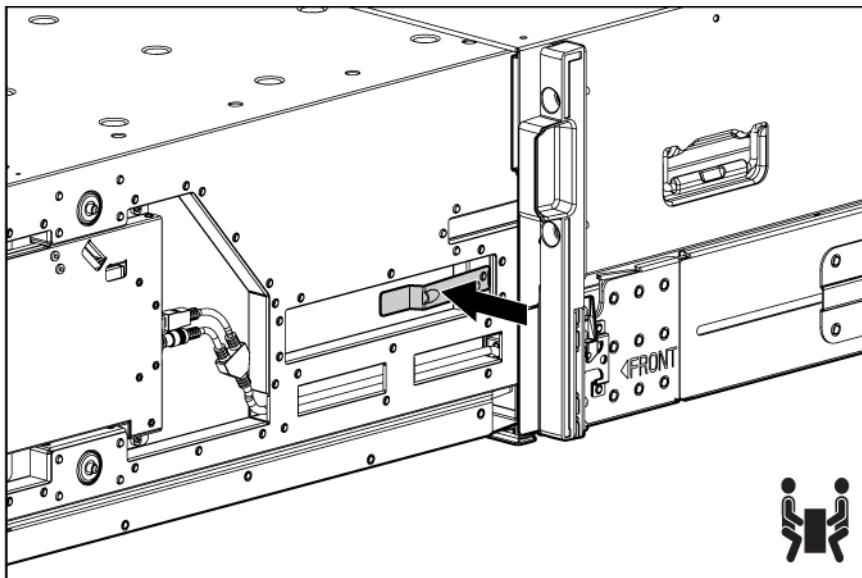
**⚠ WARNING:** When removing and lifting the front cage, always grasp the handholds as far forward as possible. The front end of the front cage is heavy and the handholds provide a more balanced location to distribute the weight of the cage during lifting.
