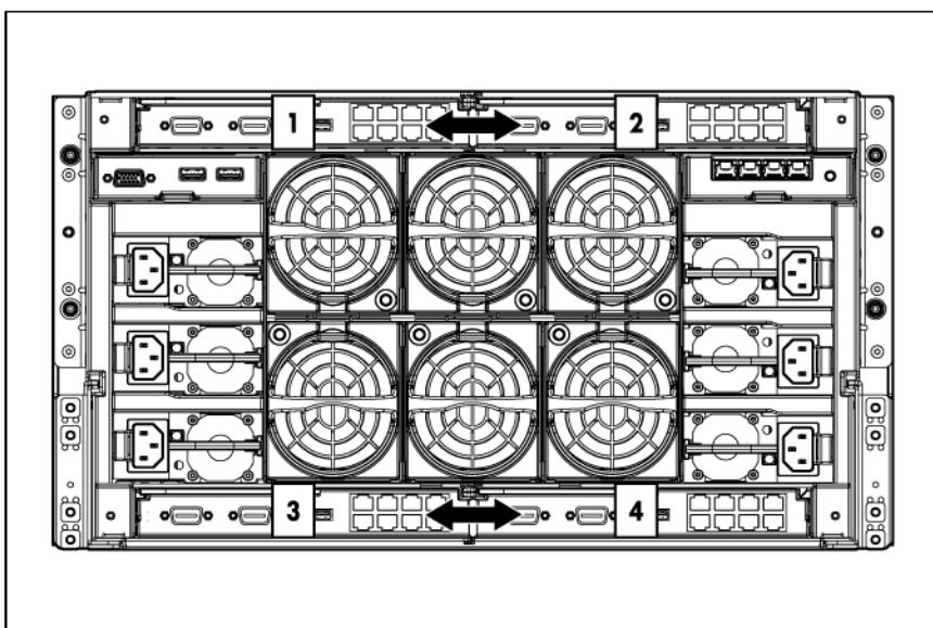
You can enable these signals to provide module-to-module connections. Onboard Administrator disables the interconnect bay crosslinks in instances where the crosslinks cannot be used, such as when two different modules reside in adjacent horizontal interconnect bays.
