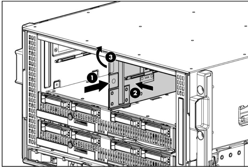
For the mini divider, push the divider toward the back of the enclosure until the divider drops out of the chassis.
