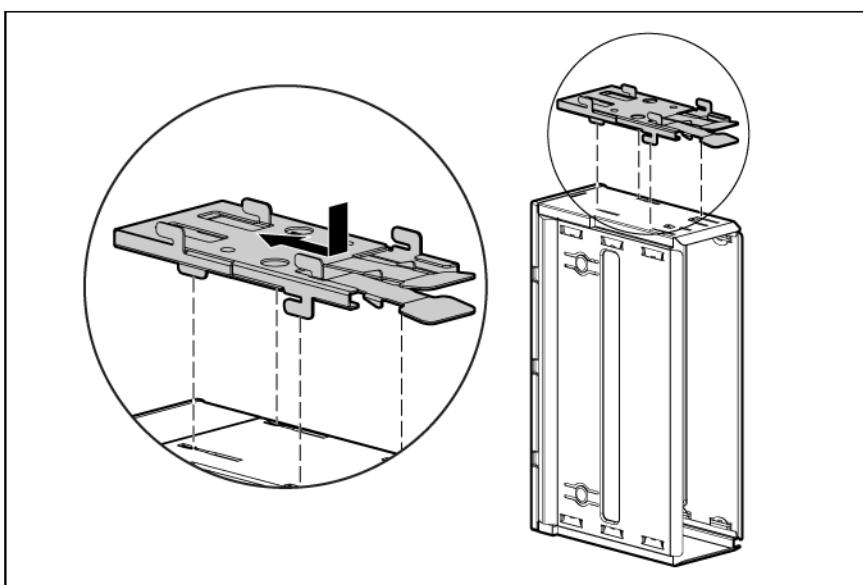
3. Fit the slots on the bottom of the second blank on to the tabs on the coupler plate, and then slide the second blank forward until it snaps in place.
