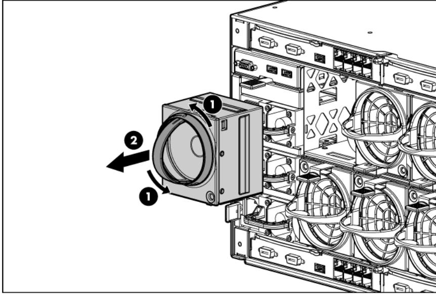
2. Slide the fan into the enclosure until it locks in place.
