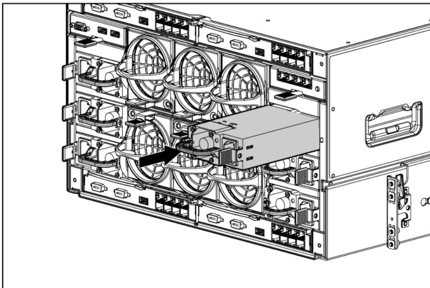
**NOTE:** When installing a power supply in power supply bay 1, 2, or 3, orient the power supply so the plug is on the left side. When installing a power supply in power supply bay 4, 5, or 6, orient the power supply so the plug is on the right side.
