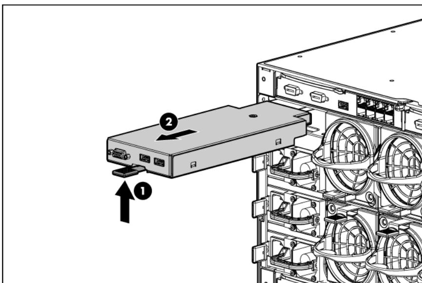
3. Install a blank in an unused KVM module bay. When fully inserted, the device locks into place.
