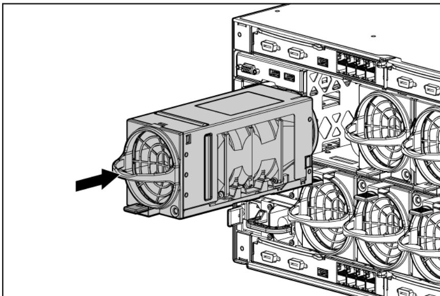
To remove a fan, turn the handle counterclockwise to the unlock position, and pull the fan out of the enclosure.
