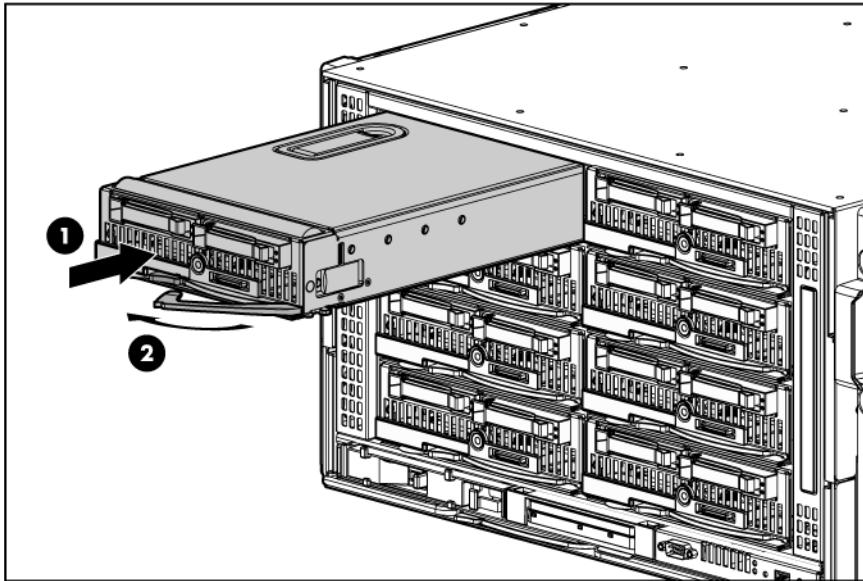
**NOTE:** If you plan to install four Active Cool 100 Fans, you can install up to four half-height blades. Populate the device bays in the following order: 1, 2, 5, 6.
