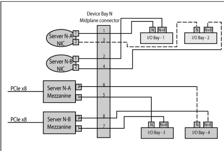
To support network connections for specific signals, install an interconnect module in the bay corresponding to the embedded NIC or mezzanine signals.
