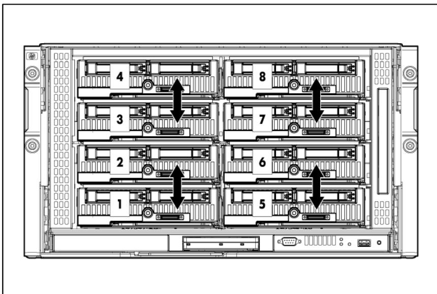
For half-height blades, these signals are used to connect a four-lane PCIe module to a partner blade such as a tape blade or a PCI expansion blade. For full-height blades, these signals are used to connect a PCIe module to a partner blade in the lower adjacent bay and require a PCIe pass-through mezzanine card installed in mezzanine connector 3. Onboard Administrator disables the device bay crosslinks in instances where they cannot be used, such as when two blades reside in adjacent device bays.
