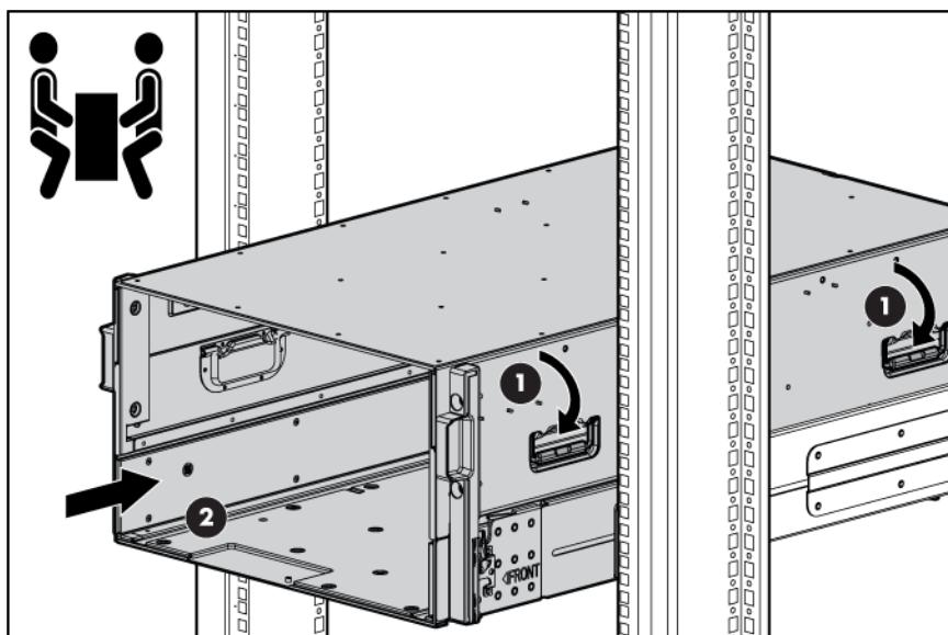
3. Tighten the thumbscrews to secure the enclosure to the rack.
