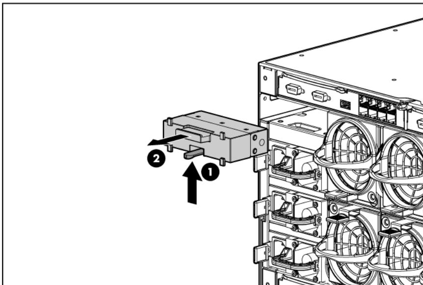
2. Slide the c3000 KVM module into the bay. When fully inserted, the device locks into place.
