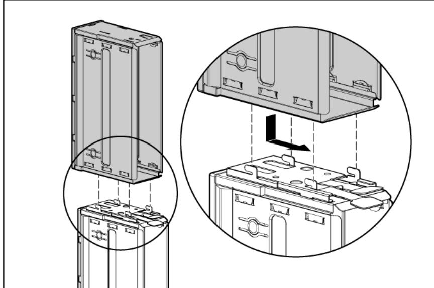
4. Install the full-height blank into the device bay.
