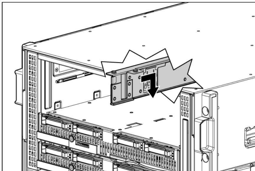
4. Remove the device bay divider from the enclosure.
