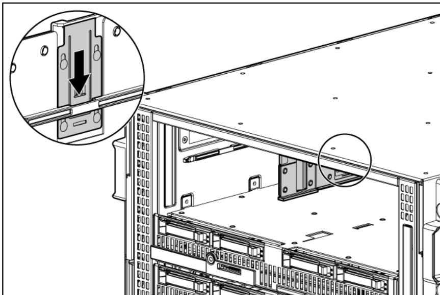
3. For the half-height divider, push the divider toward the back of the enclosure until the divider stops. Slide the divider to the left to disengage the tabs from the divider wall, and then rotate the divider clockwise.
