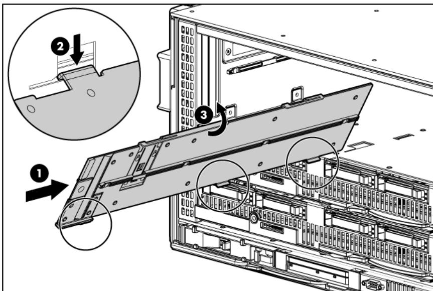
**CAUTION:** Be sure that all five tabs (three on the bottom edge of the divider and two on the top edge of the divider) are fully inserted before sliding the divider forward to complete the installation. Failure to do so can cause damage to the blade connectors during installation.
